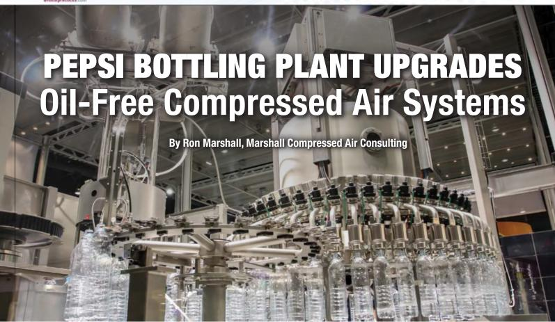
➤ The Pepsi bottling plant in Winnipeg, Manitoba has upgraded both their main 100 psi compressed air system and their 600 psi PET bottling system in two separate projects. The system improvements have saved the company both maintenance and electrical operating costs, and even reduced some winter heating demand.
