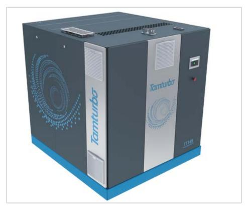
View of the Tamturbo® model TT145 3-stage active magnetic bearing air compressor.
