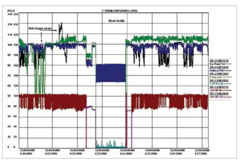
Figure 1: The as found system was found to be operating inefficiently, note how the air compressor amps fall from 70 to almost nothing when the reciprocating compressor runs.
