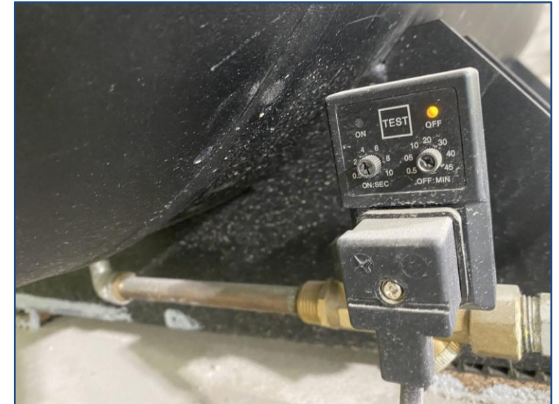
The TEST button + interval dials — a monthly press confirms it still puffs and reseals
