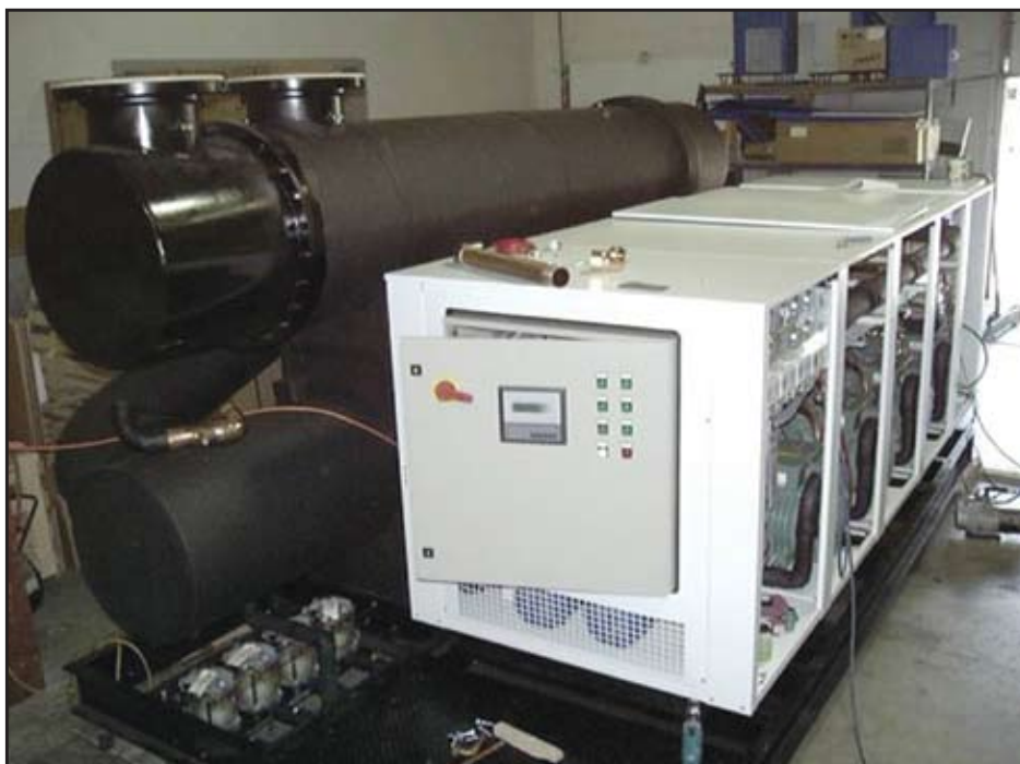
Cycling Dryer With Multiple Refrigeration Compressors
