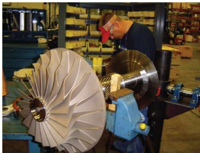
Work-in-Progress on a FS Elliott Impeller
