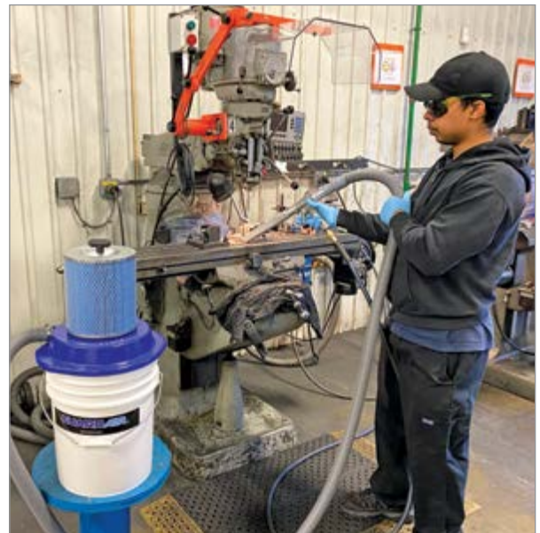
This handheld vacuum gun is connected to a 5 gallon storage container for collecting debris such as metal chips, shavings, sand, powders or sawdust.
