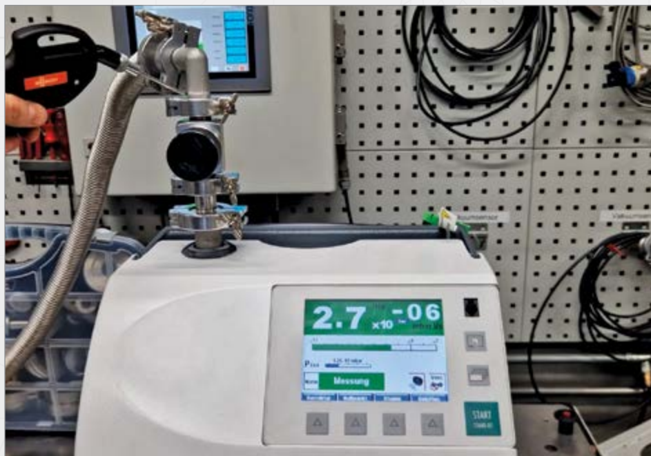
Leak detection tests must be performed in a stable environment with a consistent temperature for precise results. (Source: Busch Vacuum Solutions)
