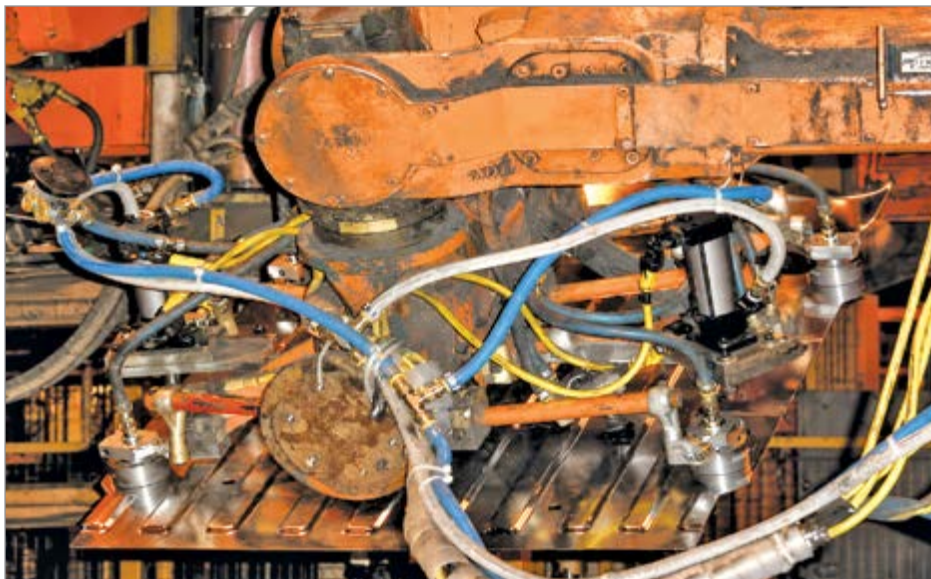
Figure 8. Four magnetic pickups replaced eight vacuum cups on this robotic end effector.
