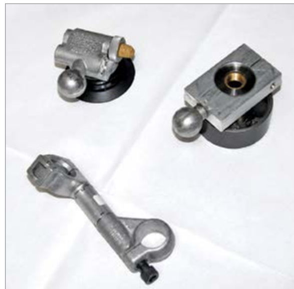
Figure 2. In this project, a vacuum cup (top left) is replaced by a spring-return magnetic pickup (top right) while retaining the existing adaptive tooling (bottom) where practical.
