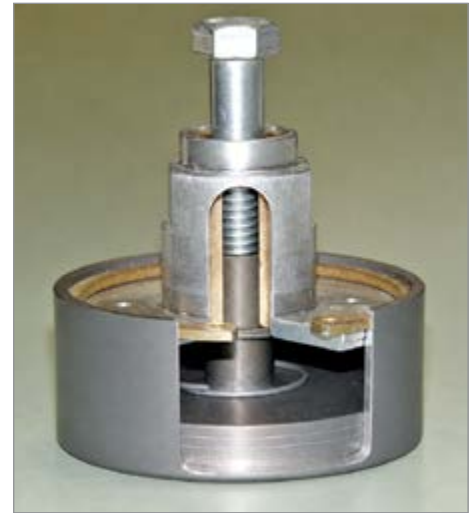
Figure 5. A cutaway view of a magnetic pickup. Compressed air at 25 psig (1.7 barg) is used for blow-off/release rather than continuous holding.
