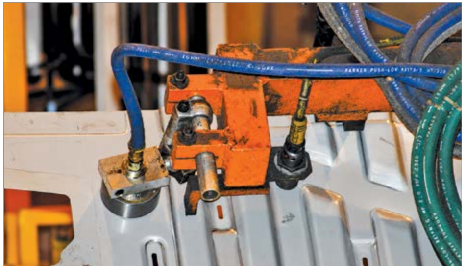
Figure 1. An overview of the end effector showing the magnetic pickup, adaptive tooling, 1 1/8-inch ball interface and compressed air release connection.
