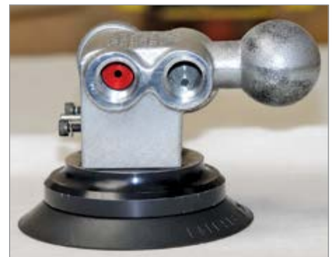
Figure 4. An existing vacuum cup and venturi assembly, including a 0.04-inch venturi orifice used on the original pneumatic pickup.
