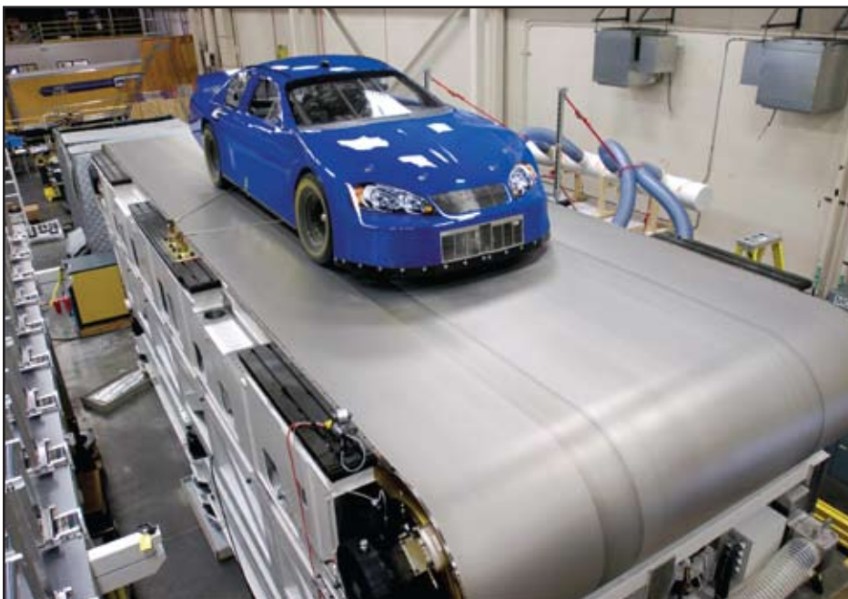
The Elevated Track Allows Race Cars to Run at 180 MPH
