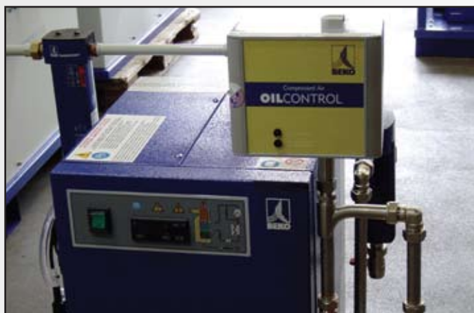
OILCONTROL instrumentation provides true measurement and alarm capabilities for oil content
