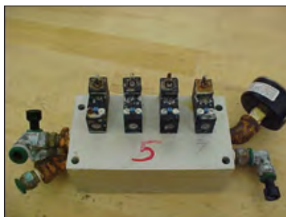
Figure 7: Kneeling module after Salt Spray Testing
