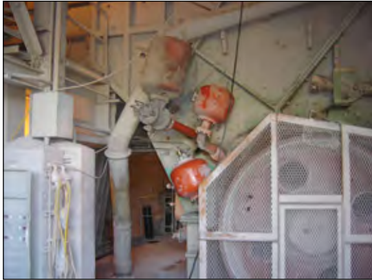
BIG BLASTER® XHV TORNADO (left) and HURRICANE Air Canons (two on right) installed on a cement plant's primary crusher.
