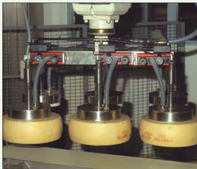
Arla Foods implemented PIAB's P6010 vacuum pumps equipped with PIAB Cruise Control (PCC) into its existing equipment to reduce air consumption by 53%.
