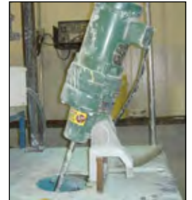
Electric motors can replace air motors for stirring.
