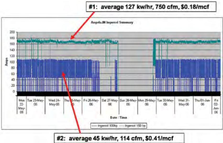
Graph showing a partially loaded compressor and a fully loaded compressor.
