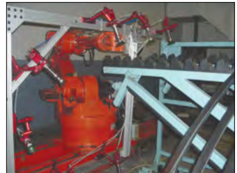
PIAB's COAX® multistage ejectors achieved an evacuation flow rate of 85 scfh and produced a holding force of 100 lbs, which is 25% higher than competitors' solutions used in the study.
