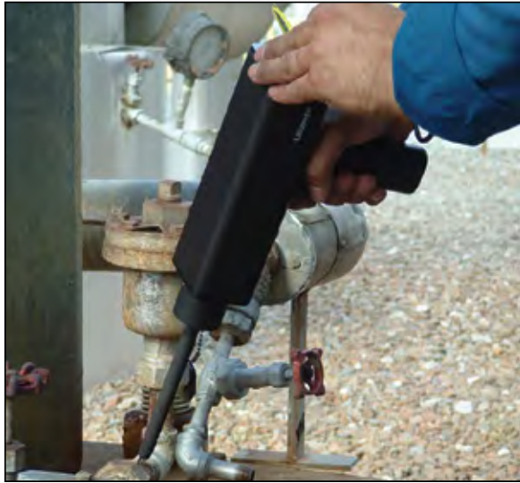
A 600 psi-rated steam trap being ultrasonically tested
