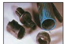
Figure 9. Represents a factory air system. A typical system consists of compressor(s), controls and regulators, dryer, receiver, ring main and individual users. The photographs on the right indicate corrosion and build-up from improper filter maintenance, costly and corrosive condensate from a poorly maintained dryer, and damaged tools and fittings, all of which can lead to unscheduled maintenance increased costs and inefficiencies. Source: www.energymanagertraining.com/equipment_all/compressors/1.htm
