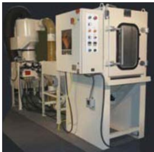
Figure 2. Typical Industrial Cabinet type sandblast unit.
