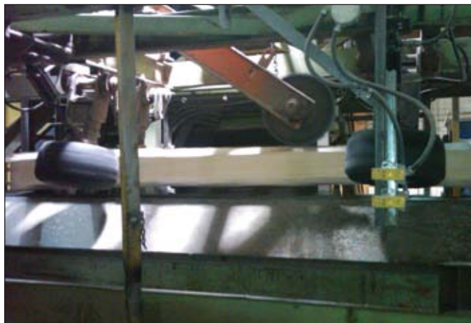
The rubber tires and overhead metal roll, of this machine center, are all air-controlled.
