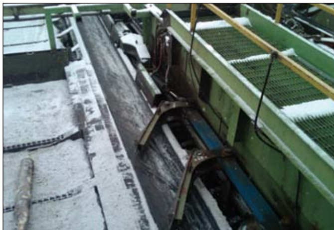
The "log kicker", at the cut-off saw station, uses air cylinders that are 8" bore x 12" stroke.
