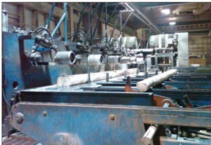
The cant optimizer infeed table positions the cant by means of air-raised positioning pins.
