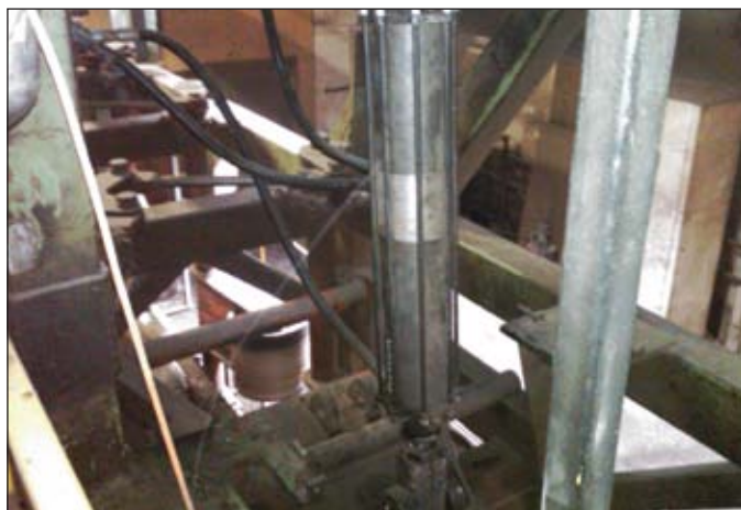
A double-piston, 6" bore cylinder impales a "sharp chain" to the logs.
