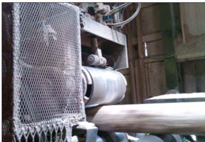
The cant optimizer outfeed rolls are controlled by air cylinders that are 6" bore x 8" stroke.
