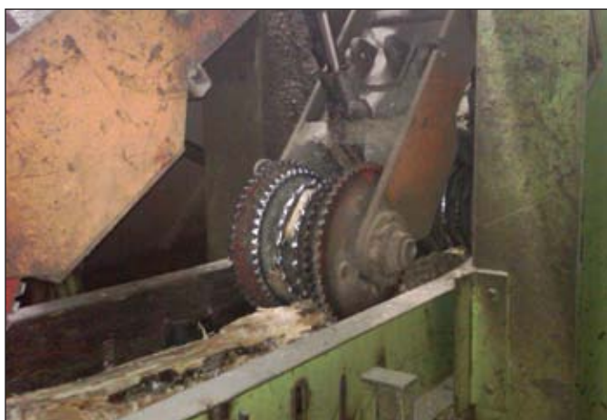
Air cylinders on the hold-down rolls of the double-length canter infeed.
