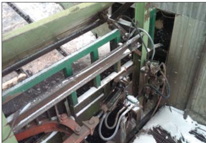
The debarker "log kicker" uses air cylinders that are 8" bore x 12" stroke and cycle 10 to 20 times per minute.
