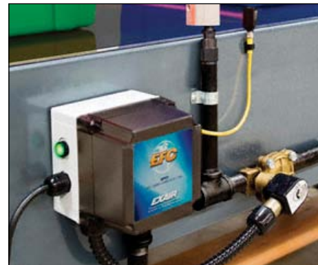
EXAIR's Electronic Flow Control minimizes compressed air use for blow off, drying, cooling, conveying and static elimination operations by turning off the air when no part is present.
