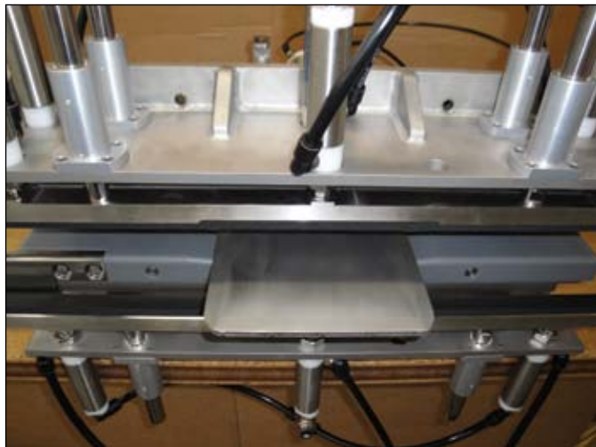
CVP Systems, Inc. developed its High-Velocity Quick-Draw Snorkel, which as part of its MasterPACKer Eco+™, provides efficient vacuum and gas insertion during the modified atmosphere packaging process.
