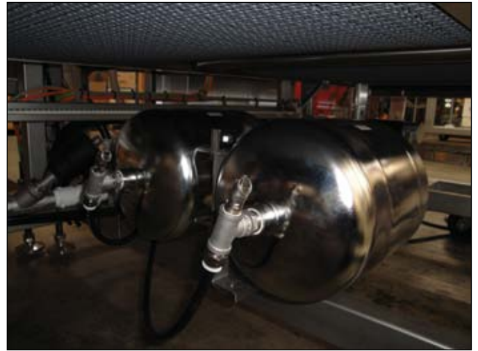
The dual gas accumulator tanks on the MasterPACKer Eco+™ are able to store on-site the application specific mixture of gas needed in the modified atmosphere packaging process.
