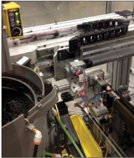
The spacers fall onto a conveying system where they are mechanically aligned by another series of pneumatic cylinders. Meanwhile, a similar process is taking place with the spools. These spools will be what eventually hold the spacers
