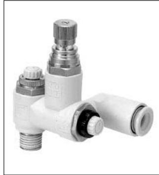
The ASQ contains an exhaust valve with a speed controller and is installed on the cylinder's high-pressure/working side.
