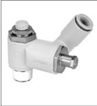
The ASR contains a regulator, check valve and speed controller and is installed on the low pressure/non-working side of the cylinder.
