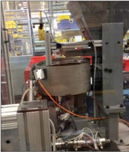
A pneumatic cylinder jolts the hopper periodically, moving the spacers to the bottom of the hopper
