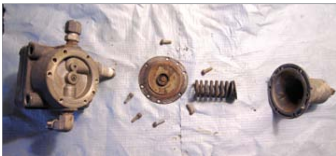
Image 1: The Components of a 1/4" Regulator.
