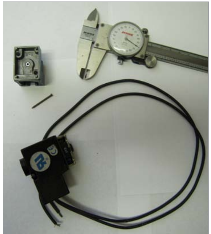
Image 8: A Common Manifold Mounted Solenoid.
