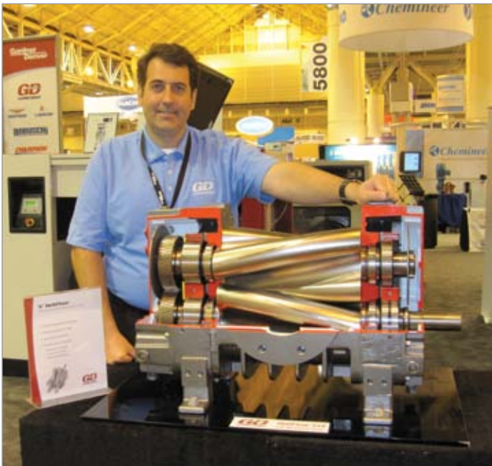
Shawn Boynton, from Gardner Denver, demonstrating the cut-away of the HeliFlow helical tri-lobe rotary blower.
