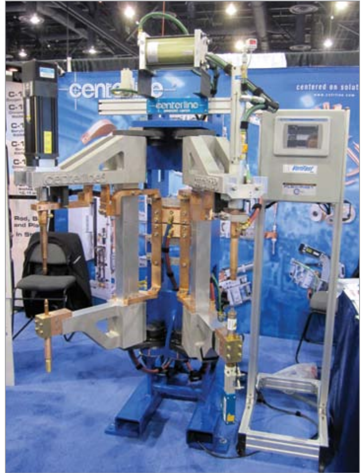
A CenterLine FlexFast™ Acrobat Welder Using Air over Oil Cylinders for Pneumatic Welding Control.
