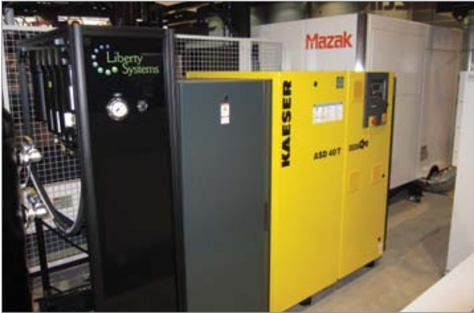
The Mazak Laser Machine Assist Gas Supply System with a Kaeser ASD Series rotary screw compressor.
