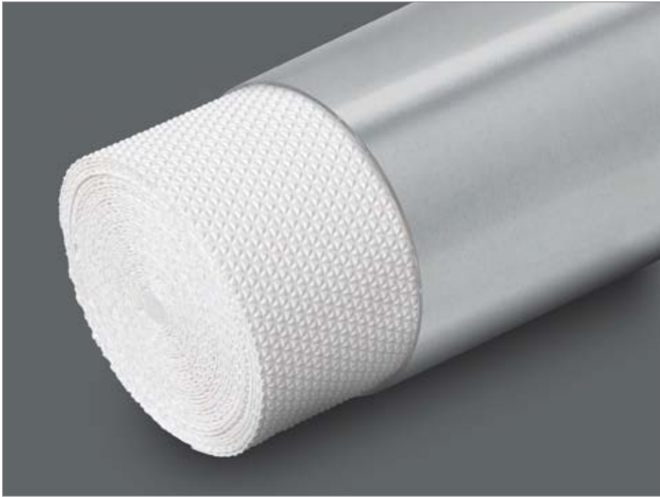
Example of Skroll medium being loaded into an aluminum tube. Internal diameter 62 mm (2.44") bore x 218 mm (8.6") long. Inlet flow capacity at 7 bar (100 psig) is 280 NI/min (10 scfm) for a 40 °C (72 °F) dew point suppression.
