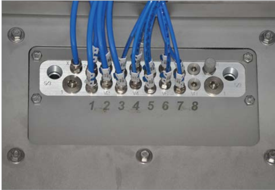
A corner strip with an all-round seal prevents the valves from coming into direct contact with H_2O_2 -impregnated air in a standard valve system.
