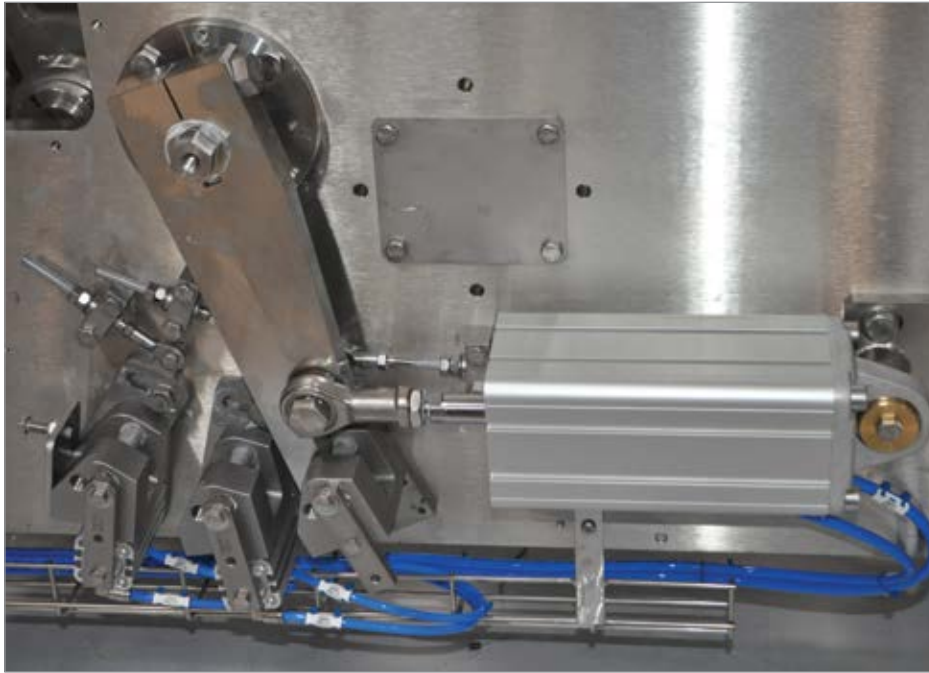
Aventics' CCI compact cylinder facilitates adjustments for packaging heights.
