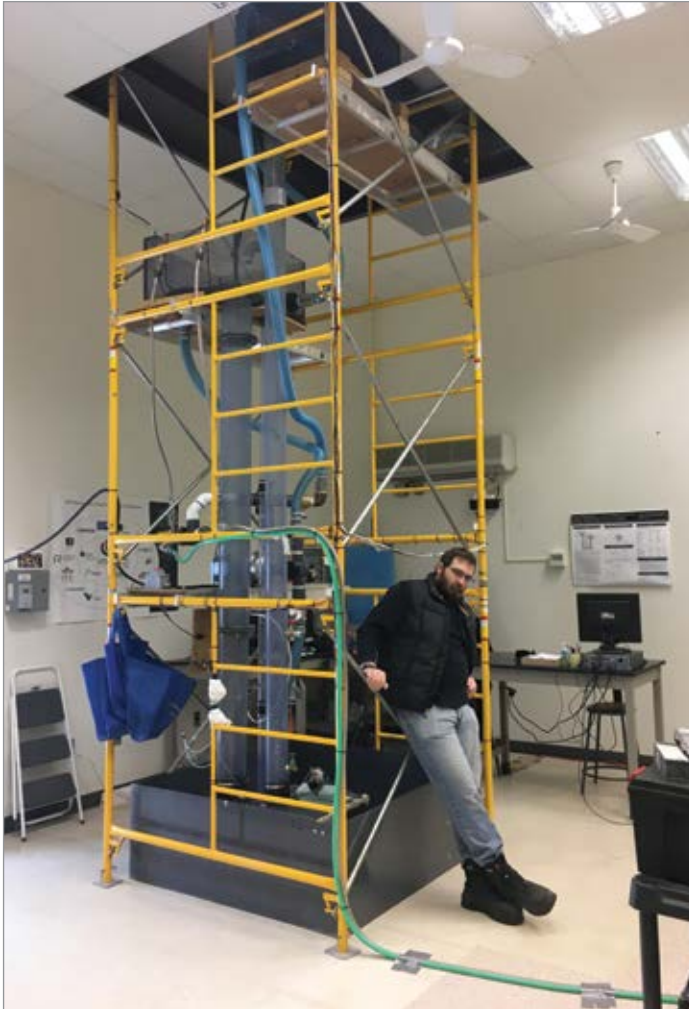
This laboratory-scale HAC, which is about 15 feet tall, is used for basic testing in a controlled environment. Alex Hutchison (pictured) is a Project Engineer with Electrale Innovation Limited. He played a key role in the development of the modern HAC.
