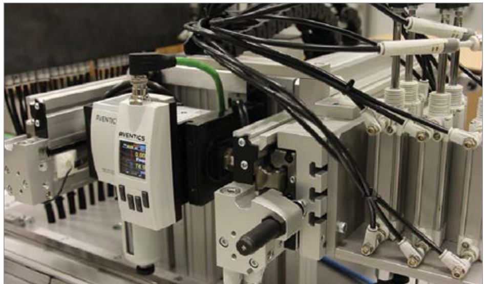
The AVENTICS Series AF2 flow sensor continuously monitors air consumption in pneumatic systems, providing actionable insights to help optimize energy consumption, prevent machine downtime, and reduce costs.
