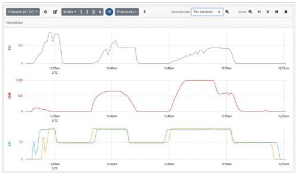
Shown is the load profile of the pressing process at the chemical plant. As shown, only the pressure sequence at 12:35 am requires high pressure air at 180 psi. Additionally, consumption of compressed air is low during this same period compared with the rest of the sequence. The short period of high pressure at 12:40 am during the purge sequence is caused by backpressure of stationary liquid. The rest of the sequence only requires compressed air at 100 psi.
