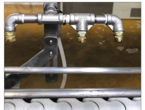
Three brass nozzles designed for spraying liquid being used improperly to blow air on a food packaging line.
