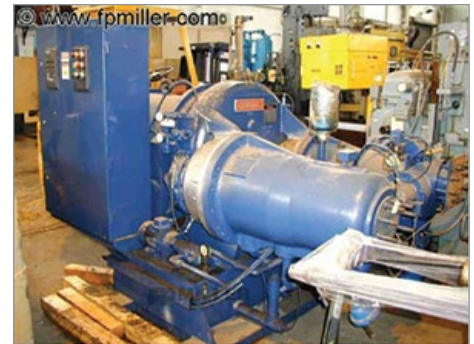
Figure 6. Centrifugal air compressor with typical crankcase or gearbox breather filter/agglomerator to stop and collect the oil mist from migration to the ambient air.
