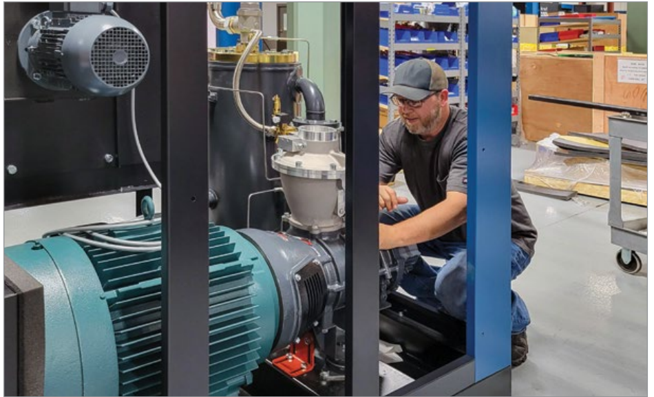
A Kaishan USA KRSP-75 fixed-speed air compressor in the process of assembly.
