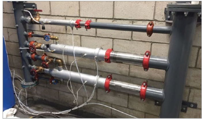
Figure 4. Sonic Nozzle Flow Measurement Application at an Air Compressor Manufacturer QA and R&D Lab (Courtesy of Hertz)
