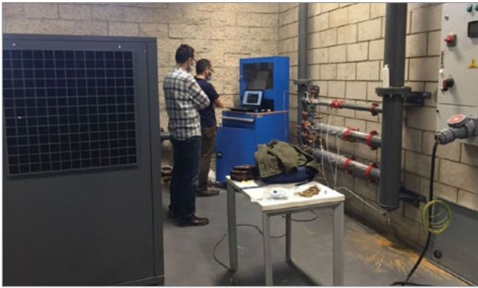
Figure 4. Sonic Nozzle Flow Measurement Application at an Air Compressor Manufacturer QA and R&D Lab (Courtesy of Hertz)
