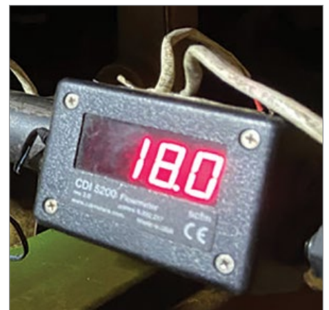
Low-cost thermal mass flow meters with wireless transmitters were used to track nitrogen consumption of the facility's three laser cutters.
