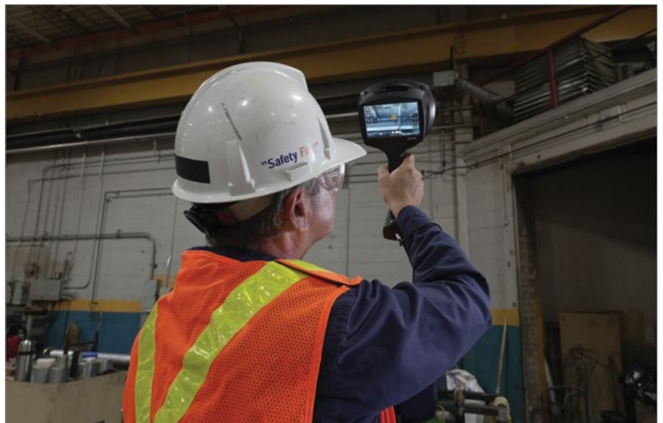
A worker conducts an inspection looking for air leaks with the FLIR Si124-LD acoustic imaging camera.
