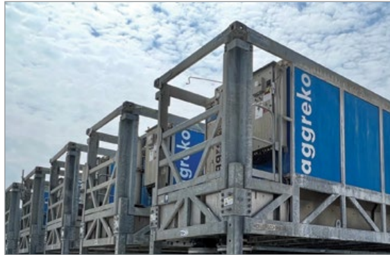
A fleet of Aggreko rental cooling tower systems.
