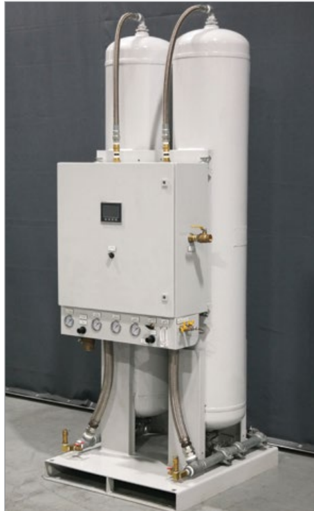
Small, twin tower PSA N_2 generator. (Note: Some designs may include multiple pairs of beds.)
