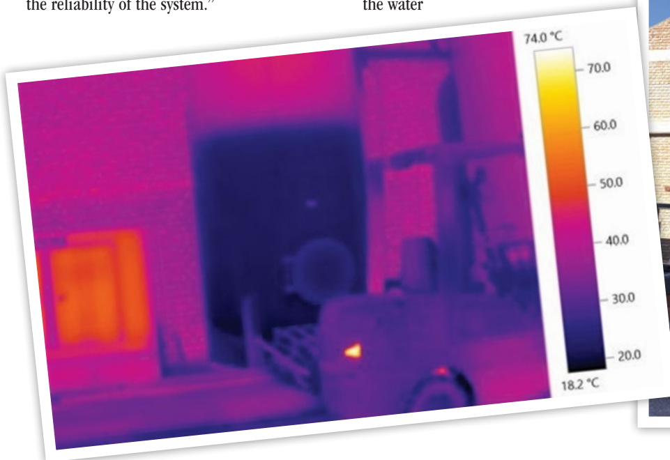
Using a thermal camera, the compressed air audit discovered the compressed air storage tank was 60% full of water. Photo credit: Marcelo Cassani, Pneumac Service S.A.
