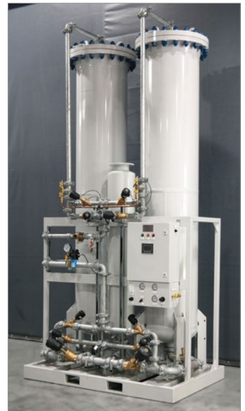
Mid-sized PSA N_2 generator as often used for laser cutting operations – produces 5700 SCFH of 99.99% N_2 (less than 100 ppm of O_2 ).
