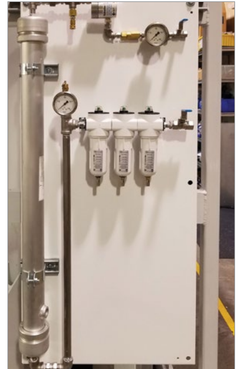
Wall-mounted membrane N_2 generator, such as might be used for dispensing beer.
