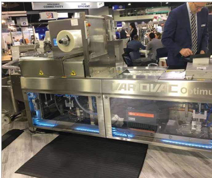
The Reiser VARIOVAC Optimus featured a rotary vane vacuum pump and compressed air inlet filtration.
