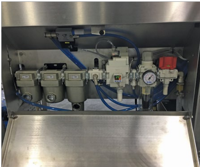
Jeff Iocco at the Sealed Air Cryovac booth. Their units feature compressed air filtration, regulation and flow measurement.
