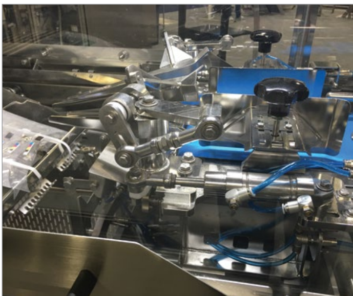
Compressed air blows directly into a bag to open it before being filled with product.
