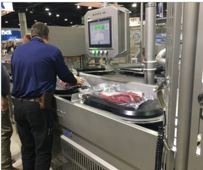
The AMCOR MODA VAC with DSS + V supported by rotary screw vacuum pumps.
